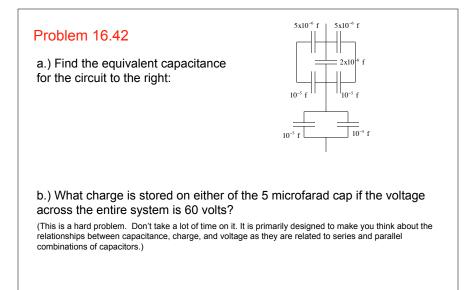
b.) What charge is stored on either of the 5 microfarad caps if the voltage across the whole combination is 60 volts?
