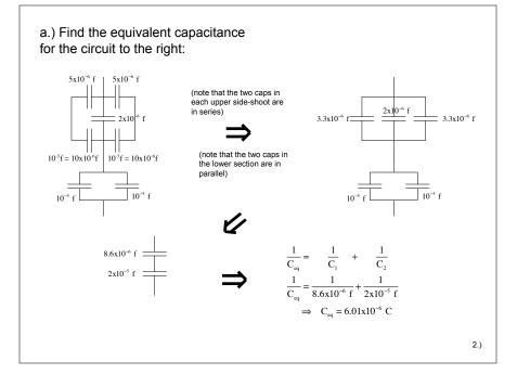
Why have I done this? Because if we can determine how much charge is associated with the  $3.3 \,\mu f$ equivalent capacitance, we will know the charge on each of the actual caps making up that section including that of  $5 \,\mu f$  cap.
